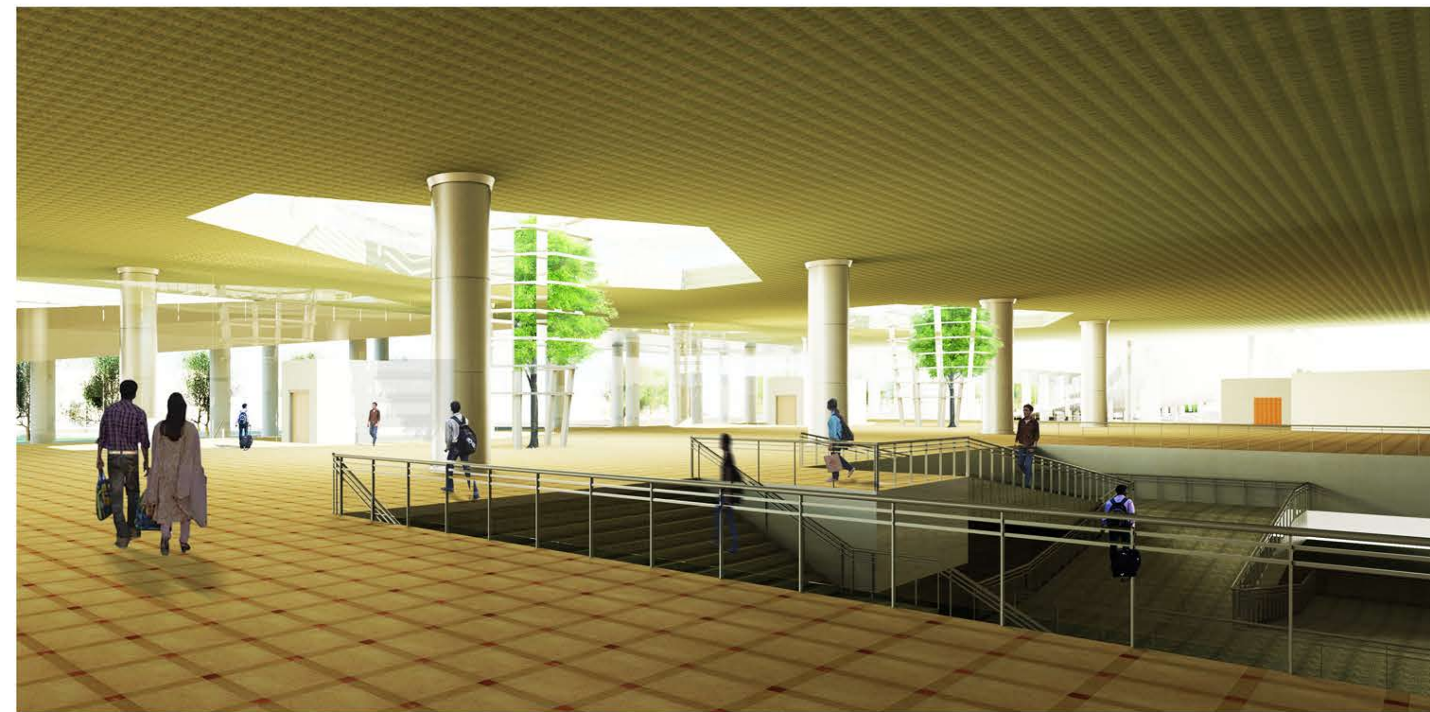
View of Arrival hall and subway. Subway is used by arriving passengers for exiting the platform and connect to the take off lane and to arrival waiting hall. It is daylighted by the cut outs in departure hall.
